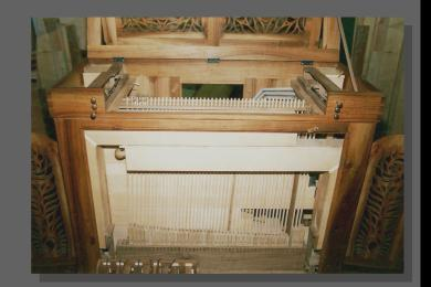
THE WIND OF ALL THE PIPES OUTSIDE THE WIND CHEST IS CARRIED BY LEAD CONDUITS.
