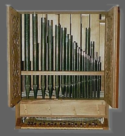
THE INSTRUMENT IS DIVIDED INTO THREE PARTS: THE TABLE CONTAINING THE BLOWER, THE CABINET CONTAINING THE PIPES, THE COPING CONTAINING THE BELLOWS. ORNAMENTAL MOTIFS
